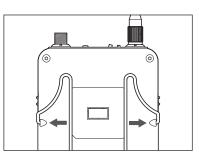
Pull both sides of the clip firmly to the outside to remove the clip from the product.
