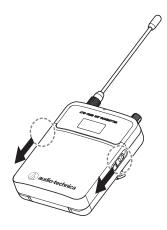
2. Open the battery cover while the latches are slid.
